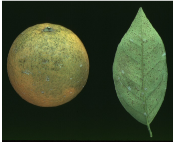
Fig. 32. Copper damage to 'Valencia' fruit and leaves caused by a copper spray. From T.W. Embleton.
